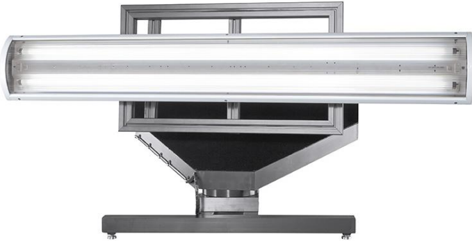
Fig. 2. The two-axis goniometer used allows the measurement of light sources that extend outside of the boundaries of the frame so that light tubes and panels can also be measured directly.
